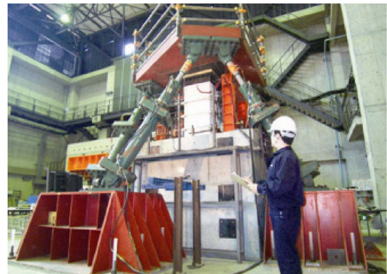
Fig. 3 Structural test for adopting high strength reinforcement (verification of seismic resistance)
