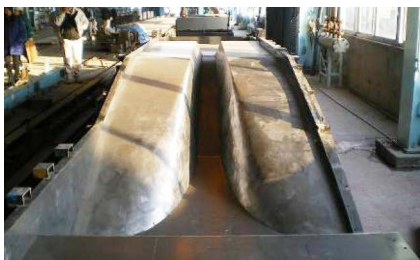
Fig. 11 Steel form for PCaPC slabs
